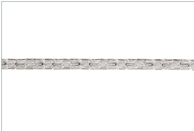
Figure 5: EluNIR Ridaforolimus DES (Medinol, Tel Aviv, Israel), laser-cut from a cobalt-chromium plate, with elastomeric coating with ridaforolimus, welded into a tube with WiZeCell cell architecture (Medinol, Tel Aviv, Israel), a hybrid between open and closed architecture. Unexpanded on carrying balloon. Images from our own archive.
